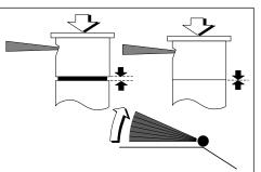
**5**. Check new arc. Adjustment made in step 4 will be added to right side of arc.
